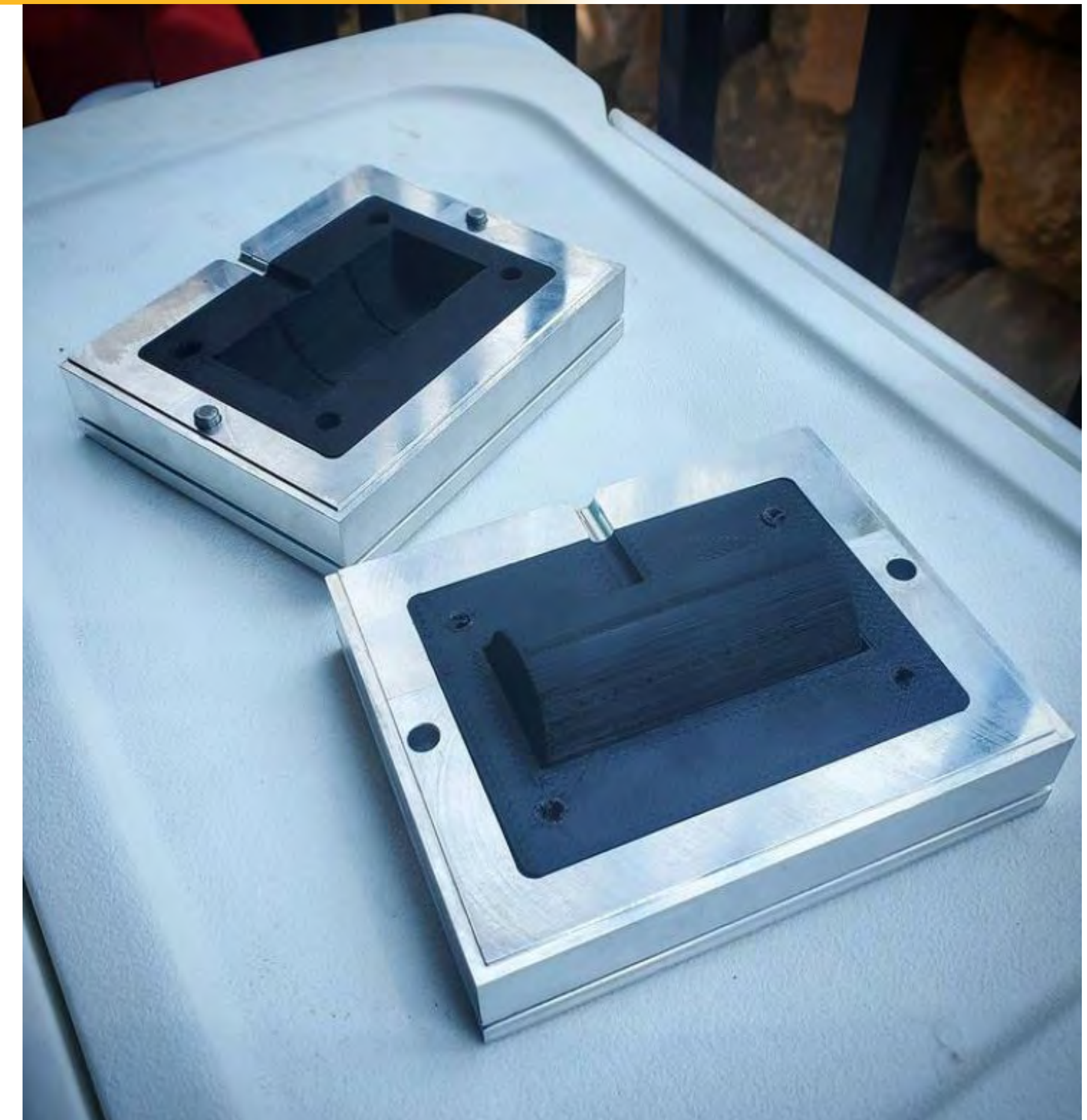
3D PRINTED INJECTION MOLDS(FINAL MOLDS ARE ALUMINUM)
